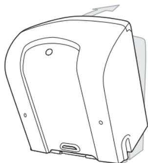
8. Push the scanner towards the plastic tab and rotate it so that it is perpendicular to the mounting surface.
